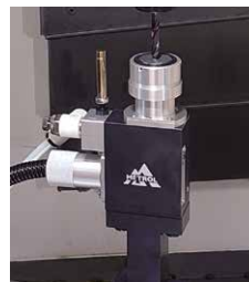
Tool length switch for automatic measurement
