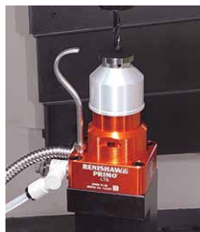
Tool length switch for automatic measurement
